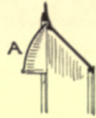
Fig. 65.—Hood inserted in Register-grate.
